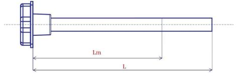
Figure 4 illustrates the original length (L) of the sensor probe and the length
