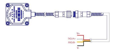
Figure 11. Wiring diagram of RS485 and RS232 output signals
