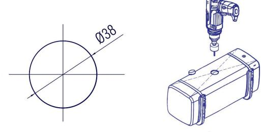
Figure 2. Drilling the selected hole
