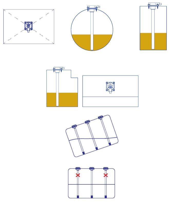
Figure 1.Selecting the location to install sensor
