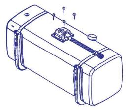
Figure 10 . Put sensor into the tank
