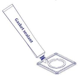
Figure 9. Applying the sealant to gasket
