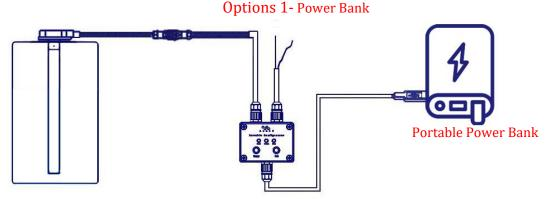
Figure 5. Connect the portable configurator USB to the power bank, and use the power bank to power the fuel level sensor.
