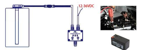
Figure 7. Portable configurator power cable connected to truck battery or battery
