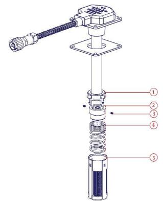
Figure 8 . Procedure for Installing the Screen Filter
