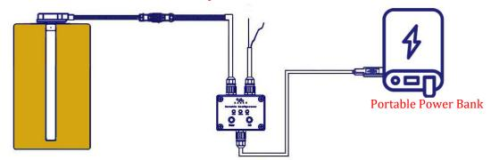
Figure 5. Connect the portable configurator USB to the power bank, and use the power bank to power the fuel level sensor.
